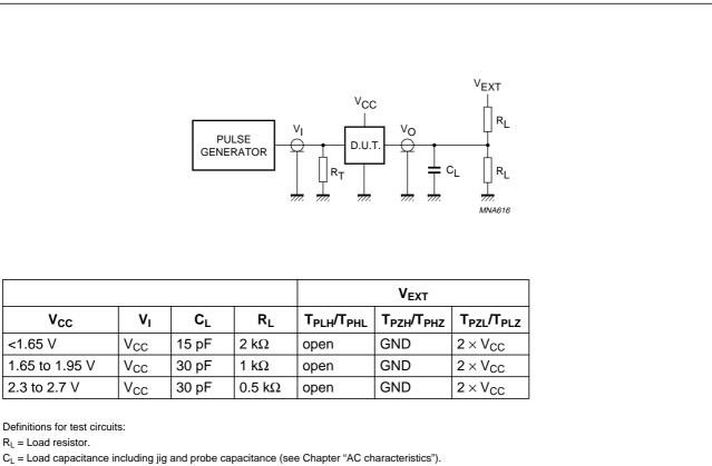
$R_T$  = Termination resistance should be equal to the output impedance  $Z_0$  of the pulse generator.
